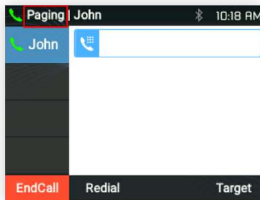
Figure 21: Call using Paging/Intercom
